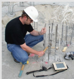
Dynamic pile integrity test
